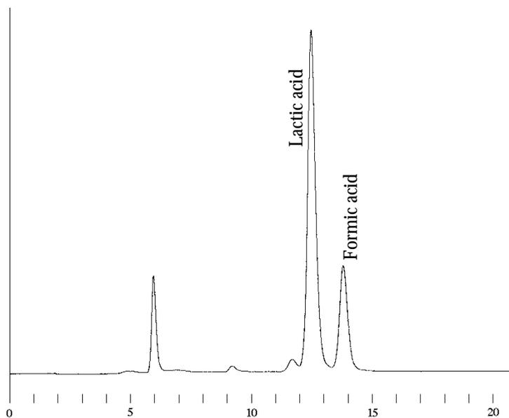
**Figure 3.** HPLC-curve with lactic acid, formic acid as internal standard
