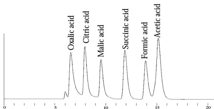
**Figure 2.** HPLC standard curve
