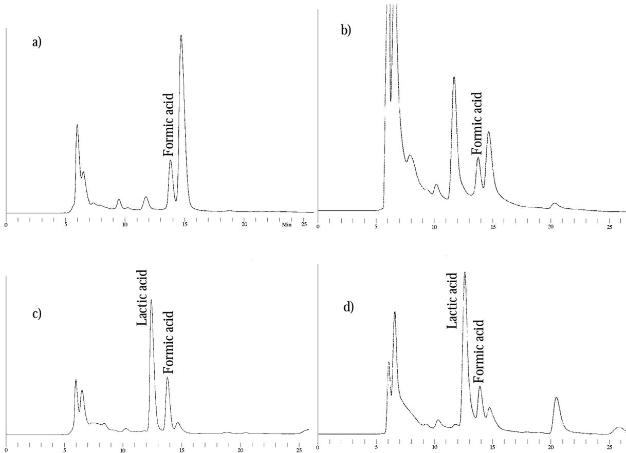
**Figure 4.** HPLC-curves, a) nonfermented bagerivetemjöl, b) nonfermented tef, c) fermented bagerivetemjöl, d) fermented tef.
